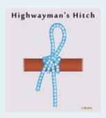
This quick release knot is of the draw loop type and can temporarily secure a load that is to be released cleanly and easily. It can be tied at the middle of a rope eliminating the need of the working end to be passed around the anchor while tying or releasing. It involves 3 bights of the same rope each of which successively lock the previous one as is evident from the below diagram. The name of the knot is attributed to Dick Turpin, a notorious 18<sup>th</sup> century English highwayman
